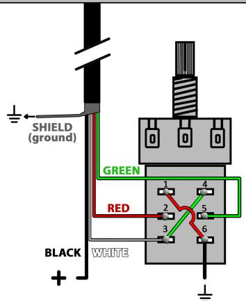
Use of a DPDT switch allows one of the two coils to be reversed to maintain full hum-cancellation and phase compatibility when combined with Lollar neck pickups. Pickup is wired in series to allow it to hum-cancel when used by itself (with switch pushed in) and also be in phase and hum-cancel when combined with the neck pickup (with the switch pulled out).
