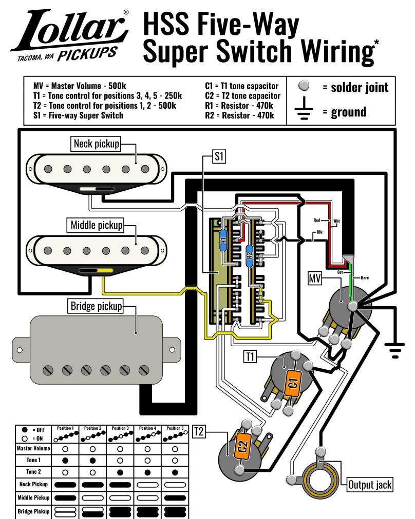
\*For Lollar Single-coil Pickups With Pushback Wire and Humbucker Pickups With Four-Conductor Wire
