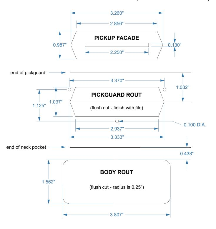
rout depth: approximately 0.938" mounting screws: #3-48 x 1.25" springs: 1.25"
