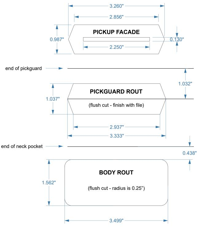
rout depth: approximately 0.938" mounting screws: #4 - 0.875" springs: 1.25"
